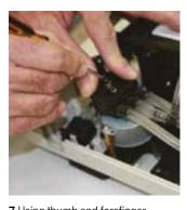
7 Using thumb and forefinger, push down firmly on the plastic rotovalve casing to release tension while removing the split pin — a deal of downward pressure is required. While maintaining downward pressure, take a small screwdriver or other implement to gently lift the split pin from the top of the motor shaft. Place the pin in a safe place for future replacement.
