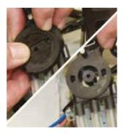
16 If the top plastic casing of the rotovalve has come lose, reposition it and hold firmly in place before replacing the rotovalve over the shaft, while sliding the 'L' shaped bracket through the plastic handle at the side of the rotovalve.
