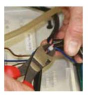
5 Using Wire Clippers (or a sharp knife) carefully cut and remove the cable tie securing the power leads between the two halves of the unit.
