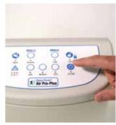
1 Switch off power supply to the Control Unit, disconnect the Air Hoses and remove the power cord from the electrical socket in the base of the unit.
