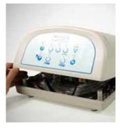
17 Align the top and bottom housing before slowly pushing closed. Ensure the seal is properly aligned around the housing, including the air hose connectors, fuses and power connector.
