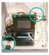
16 Before closing the housing, make sure all power leads and hoses are free from the side edges. Ensure the regulator tubing will not kink when the top cover is closed.
