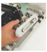
**6** Detach both internal air hoses from the inside of the Connector Plate and slide the damaged plate from the side of the unit. Dispose of the Connector Plate in an environmentally safe manner.
