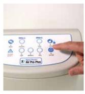
19 Test the motor before closing the housing. Connect the Control Unit to mains power and switch on to ensure the motor works and rotovalve is turning (with no adverse noise). It the Control Unit fails to operate, the unit needs to be returned to the Manufacturer for further repair or replacement. Switch off power supply to the Control Unit before closing the housing. Return the Control Unit to the manufacturer in line with standard procedures.
