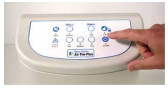
6 Reconnect the power cord to the Control Unit and switch on power supply.
