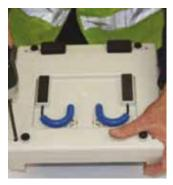
11 Using the Phillips Head Screwdriver to replace the four screws plus washers and tighten to secure the housing together.
