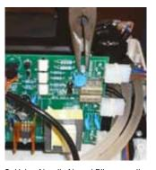
9 Using Needle Nosed Pliers, unclip the PCB from the top housing. Note the orientation of the PCB before removing it from the unit.
