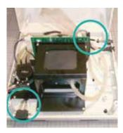
8 Before closing the housing, make sure all power leads and hoses are free from the side edges.
