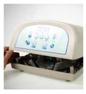
4 Gently loosen the top and bottom housing. Once loose, hold the power socket (IEC connector) to prevent from catching while lifting the top cover and leaning it back on your work surface.
