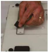
**3** Gently peel back the two foam mounting strips to reveal the plastic housing beneath.
