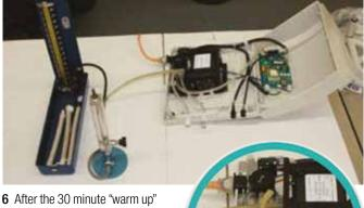
period has elapsed, detach the internal air hose from the compressor (some force may be required) and replace with the air hose from the Pressure Test Equipment (for directly connection to the compressor). Push the air hose firmly until it fully covers the connector.
