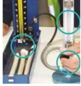
a Ensure the equipment is set to 'free flow mode' (i.e. no resistance or back pressure against the full flow of air from the compressor). The valve at the front of the Air Flow Meter should be fully open. If not, turn clockwise to open the valve to maximum. With the system in free flow mode, the ball bearing inside the Air Flow Meter should rise to a minimum of 4.5+ litres per minute. The Sphygmomanometer pressure reading should be low (approximately 10 mmHg).
