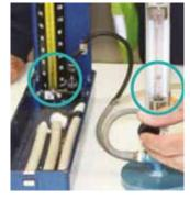
b Slowly close the valve on the Air Flow Meter to reduce airflow air and simulate 'back pressure' (i.e. to emulate the weight of a patient lying on the mattress, which forces pressure back against the flow of air from the unit). Slowly close the valve until the Sphygmomanometer pressure reading reaches 30 mmHg. At 30 mmHg, the ball bearing inside the Air Flow Meter should drop to a minimum of 3+ litres per minute.
