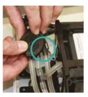
8 Gently lift the plastic rotovalve up and over the shaft, sliding the 'L' shaped metal bracket through the black plastic handle at the side of the rotovalve, to reveal the spring and synchronous motor beneath.
