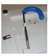
**6** Unpack the replacement hook and lay in position over the plastic bracket
