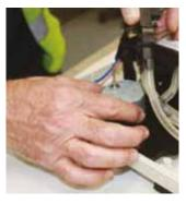
11 Lift the motor off its mounts and remove, ensuring the power lead does not get caught in the process. Dispose of the faulty motor in an environmentally safe manner.
