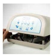
4 Gently loosen the top and bottom housing. Once loose, hold the power socket (IEC connector) to prevent from catching while lifting the top cover and leaning it back on your work surface. Be careful not to drag the internal wires and tubing during this process. Before continuing, ensure no electrical leads are stretched and that all electrical connectors on the Printed Circuit Board (PCB) are firmly connected. You may need to prop the top housing case to prevent strain on the electrical cords.
