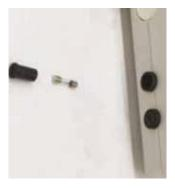
5 Insert a new fuse (or the undamaged fuse) into the plug. Push against the force of the spring and turn clockwise with the screwdriver (quarter turn).
