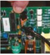
**10** Unpack the replacement PCB. Align the circuit board against the four holes and carefully reconnect the clips by pressing firmly into place.
