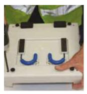
3 Use a Phillips Head Screwdriver to remove the four screws that secure the housing. Place the screws and washers in a safe place (such as small container or jar) to prevent loss. Hold the unit firmly and turn it over, face upwards on its base.
