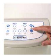
5 Reconnect the Control Unit to mains power and switch on. The unit must run for a minimum of 30 minutes to "warm up" before pressure testing commences.
