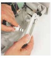
3 Insert the replacement connector (male or female as appropriate) and turn clockwise to tighten until firm.
