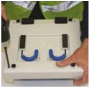
**3** Using a suitable tool (such as 2mm flat head screwdriver), gently press the clip on each air filter cover to remove.
