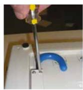
**9** Replace the plastic housing and use the Phillips Head Screwdriver to replace the three screws to secure.
