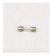
4 Visually inspect the fuse — check if the metal filament inside the fuse cylinder is disconnected or snapped — and discard if damaged (or re-insert if undamaged).
