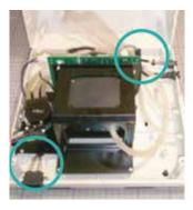
20 Before closing the housing, make sure all power leads and hoses are free from the side edges. Ensure the regulator tubing will not kink when the top cover is closed.
