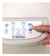
8 Reconnect mains power, switch on the Control Unit and check the Display Panel. If the unit now operates, the internal PCB has failed and needs replacing. Proceed to the Printed Circuit Board Replacement procedure for next steps.
