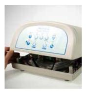
10 Align the top and bottom housing before slowly pushing closed. Ensure the seal is properly aligned around the housing, including the air hose connectors, fuses and power connector.
