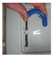
7 Slide the hook into the spring and push the hook into the base mount.
