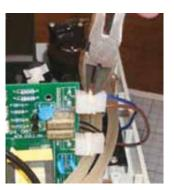
5 Disconnect the four electronic power leads by cutting the cable ties that secure the leads to the PCB. Carefully pull the plastic casing (not the wiring) to disconnect.
