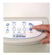
1 Switch off power supply to the Control Unit, disconnect the Air Hoses and remove the power cord from the electrical socket in the base of the unit.
