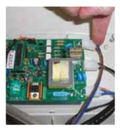
15 Reconnect the compressor power lead to the circuit board and attach a new cable tie to secure all power leads as before.
