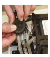
14 To test correct alignment of the motor and bracket, insert both bolts to secure the motor but finger tighten only. Gently place the rotovalve over the shaft to check the 'L' shaped bracket is correctly positioned to slide through the plastic handle at the side of the rotovalve. Once alignment is verified, remove the rotovalve and using the 7/32 inch socket wrench, tighten both bolts to firmly secure the motor in place. Be careful not to overtighten.
