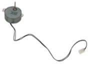
12 Unpack the replacement motor. Carefully thread the power lead under the base of the compressor cage before repositioning the new motor over the shaft and on its mounts, ensuring bolt holes are correctly aligned.
