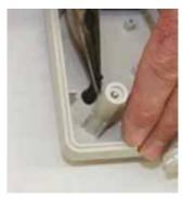
8 Once through the hole, lay the bottom housing flat and use the Needle Nose Pliers to gently pull through until the rim of the foot locks into place. Move gently from side to side while pulling, rather than applying direct upward force, to avoid snapping the nose of the replacement foot.
