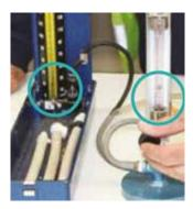
c Continue to increase back pressure resistance. Slowly close the valve on the Air Flow Meter until the Sphygmomanometer pressure reading reaches 60 mmHg. At 60 mmHg, the ball bearing inside the Air Flow Meter should drop to a minimum of 2+ litres per minute.
