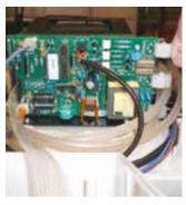
6 Disconnect the remaining three connections from the PCB (two flat digital leads and one air tube). Be sure to note the location of all seven connections on the circuit board for easy replacement.
