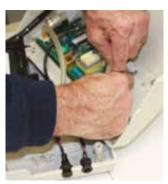
6 Trace the power lead running from underneath the synchronous motor to its connection on the circuit board. Disconnect this lead from the circuit board by carefully pulling the plastic casing (not the wiring) and gently remove the lead from under the compressor cage and leave it free.
