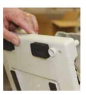
6 Lift the bottom housing up to access the base of the unit. For damaged feet, use the Needle Nose Pliers to hold the rubber base and remove from the casing.
