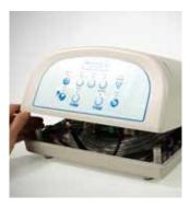
9 Align the top and bottom housing before slowly pushing closed.
