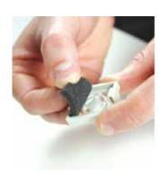
4 Remove each foam air filter for cleaning or replacement. The foam air filters and filter casings may be washed with soap and water. Rinse with plain water and dry thoroughly before returning to the Control Unit. Alternatively refit with a new filter (recommended annually).
