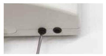
2 Using a level surface, place the Control Unit on its base, with easy access to the black round fuse cap located on the side of the unit (closest to the connectors).
