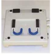
10 Holding the top and bottom housing firmly together, turn the Control Unit upside down, with base facing upwards.
