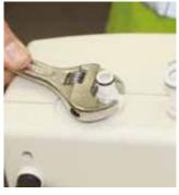
2 Using an Adjustable Wrench, unscrew the damaged quick-release connector from the side of the unit by turning it counterclockwise — a degree of force may be required to initially loosen the connector.
