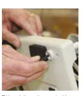
7 Unpack the replacement rubber feet. Insert the long nose of the rubber foot into the empty socket on the base of the unit (pushing from outside in).
