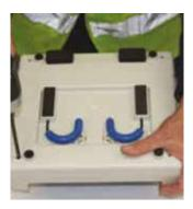
19 Use a Phillips Head Screwdriver to replace the four screws plus washers and tighten to secure the housing together.
