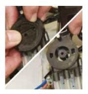
The rotovalve is made of two plastic circular casings held together by lubricant material, and should remain attached during removal. If the top casing comes free during this process, place in a safe place until time to replace the rotovalve, when it can be reattached.
