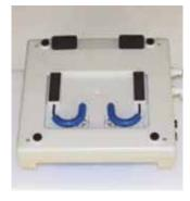
18 Holding the top and bottom housing firmly together, turn the Control Unit upside down, with base facing upwards.
