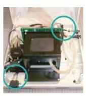
9 Before closing the housing, make sure all power leads and hoses are free from the side edges. Ensure the regulator tubing will not kink when the top cover is closed.
