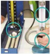
d Finish testing by fully closing the Air Flow Meter valve (maximum resistance). The ball bearing inside the Air Flow Meter should drop to 0 and the Sphygmomanometer pressure reading should rise to 120+ mmHg.
