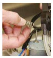
**9** Remove the spring and place it in a safe place for future replacement.
