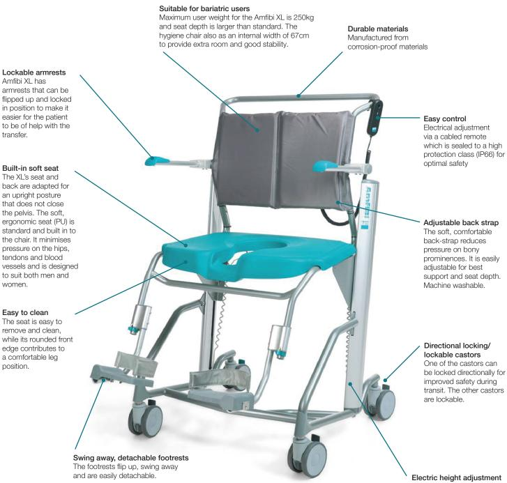
Amfibi XL has a unique pillar design for quick and easy seat height adjustment. The seat can be raised by up to 81cm from its lowest position and thus requires minimised effort from care personnel.
