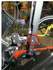
Push the backrest forward and move the actuator downwards until the bolts will appear from underneath the cover.
