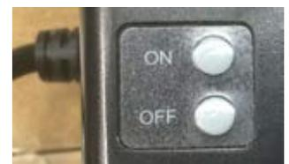
NOTE: The battery has an in-built device that automatically switches it off when remaining charge is <20%. The LED is then extinguished. The battery must now be fully charged before the electronics can be used again.
