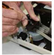
17 Firmly push down on the rotovalve while replacing the split pin through the top of the shaft. A significant amount of pressure is required to counteract the force of the spring.
