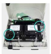
8 Before closing the housing, make sure all power leads and hoses are free from the side edges. Ensure the regulator tubing will not kink when the top cover is closed.
