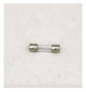
4 Visually inspect the fuse – check if the metal filament inside the fuse cylinder is disconnected or snapped – and discard if damaged (or re-insert if undamaged).
