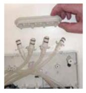
8 Unpack the replacement Connector Plate and refit all four connectors in the correct sequence, twisting clockwise to lock into place.
