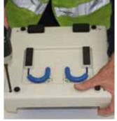
Screwdriver to replace the four screws plus washers and tighten to secure the housing together.
