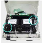
10 Reposition the Connector Plate into the side of the control unit. Before closing the housing, make sure all power leads and hoses are free from the side edges. Ensure the regulator tubing will not kink when the top cover is closed.
