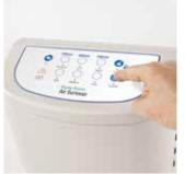
8 Reconnect mains power, switch on the Control Unit and check the Display Panel. If the unit now operates, the internal PCB has failed and needs replacing. Proceed to the Printed Circuit Board Replacement procedure for next steps.
