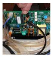
7 Take the working spare PCB and reconnect all seven leads into the corresponding connectors (four electronic leads; two digital; one air hose).
