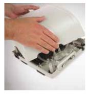
4 Gently loosen the top and bottom housing. Once loose, hold the power socket (IEC connector) to prevent from catching while lifting the top cover and leaning it back on your work surface.
