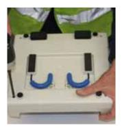
12 Using the Phillips Head Screwdriver to replace the four screws plus washers and tighten to secure the housing together.
