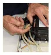
14 Reattach the air hose to the compressor, using gentle pressure to ensure a firm fit.
