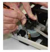
7 Using thumb and forefinger, push down firmly on the plastic rotovalve casing to release tension while removing the split pin – a deal of downward pressure is required. While maintaining downward pressure, take a small screwdriver or other implement to gently lift the split pin from the top of the motor shaft. Place the pin in a safe place for future replacement.
