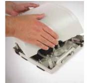
**10** Align the top and bottom housing before slowly pushing closed. Ensure the seal is properly aligned around the housing, including the air hose connectors, fuses and power connector.
