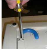
**9** Replace the plastic housing and use the Phillips Head Screwdriver to replace the three screws to secure.
