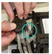
8 Gently lift the plastic rotovalve up and over the shaft, sliding the 'L' shaped metal bracket through the black plastic handle at the side of the rotovalve, to reveal the spring and synchronous motor beneath.
