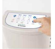
Switch off power supply to the Control Unit and remove the power cord from the electrical socket in the base of the unit before disconnecting the Pressure Test Equipment air hose.
