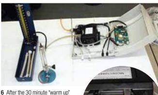
6 After the 30 minute 'warm up' period has elapsed, detach the internal air hose from the compressor (some force may be required) and replace with the air hose from the Pressure Test Equipment (for directly connection to the compressor). Push the air hose firmly until it fully covers the connector.
