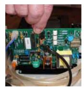
**10** Unpack the replacement PCB. Align the circuit board against the four holes and carefully reconnect the clips by pressing firmly into place.
