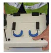
**11** Use a Phillips Head Screwdriver to replace the four screws plus washers and tighten to secure the housing together.
