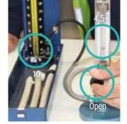
a Ensure the equipment is set to 'free flow mode' (i.e. no resistance or back pressure against the full flow of air from the compressor). The valve at the front of the Air Flow Meter should be fully open. If not, turn clockwise to open the valve to maximum. With the system in free flow mode, the ball bearing inside the Air Flow Meter should rise to a minimum of 4.5+ litres per minute. The Sphygmomanometer pressure reading should be low (approximately 10 mmHg).
