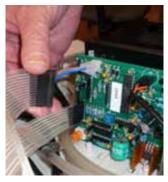
**11** Reconnect all seven leads into the corresponding connectors on the circuit board.
