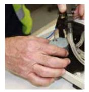
11 Lift the motor off its mounts and remove, ensuring the power lead does not get caught in the process. Dispose of the faulty motor in an environmentally safe manner.
