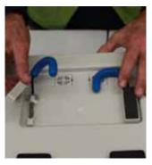
4 Use a Phillips Head screwdriver to unscrew the three screws that secure the plastic housing. Place the screws in a safe place (such as small container or jar) to prevent loss. Lift the plastic housing to reveal the spring connection.
