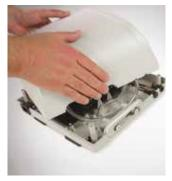
4 Gently loosen the top and bottom housing. Once loose, hold the power socket (IEC connector) to prevent from catching while lifting the top cover and leaning it back on your work surface. Be careful not to drag the internal wires and tubing during this process. Before continuing, ensure no electrical leads are stretched and that all electrical connectors on the Printed Circuit Board (PCB) are firmly connected. You may need to prop the top housing case to prevent strain on the electrical cords.
