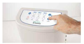
6 Reconnect the power cord to the Control Unit and switch on power supply. If Control Unit still fails to operate, the problem may be due to a faulty circuit board. Proceed to Printed Circuit Board Check procedure.
