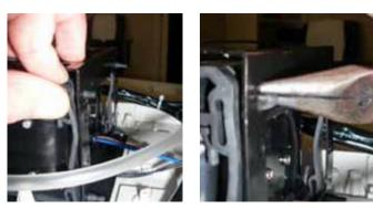
**12** Secure the compressor to the metal cage by connecting the eight new rubber mounts, starting with four mounts on one side of the cage (bottom followed by top), then four mounts on opposite side.
