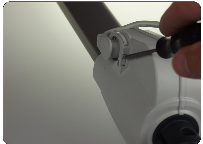
Release the locking device
