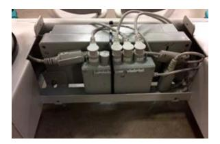
Actuators (2x up / down and 1x tilt), The actuators are connected directly to the control box as below. Remote control and battery are connected via spindle cable to control box as below.
