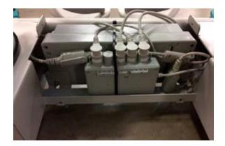
Actuators (2x up / down and 1x tilt), The actuators are connected directly to the control box as below. Remote control and battery are connected via spindle cable to control box as below.
