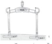
1. First, place the RoMedicClips on the slingbar by looping the suspension loops on to the slingbar hooks.
