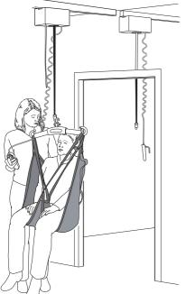
When sufficient tension has been relieved from the lift strap on lift unit 1, it can be removed from the RTH hook.
