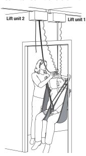
Before lifting the patient, ensure that the "empty" hook on the RTH hook is facing the doorway / the second lift unit.
