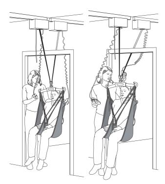
Run the lift strap into lift unit 2 so that the patient is moved through the doorway in a single, gentle motion.
