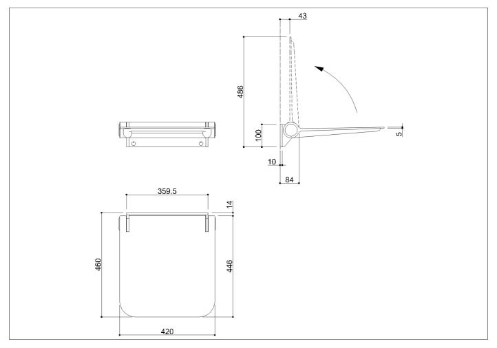
Folding seat in polyurethane with internal structure in stainless steel and fixing flange in aluminium
