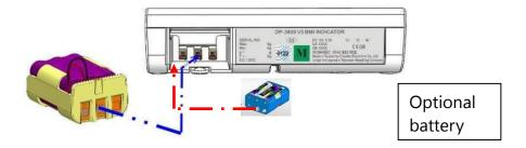
4. Place the housing back in the back of the indicator, and close the battery housing cover.
