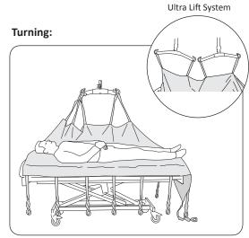
1. Disconnect the loop straps from the side nearest the centre of the bed. If SideBars have been used in the first stage, disconnect them and distribute the lift straps on the sling bar when it is hanging parallel with the bed.
