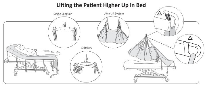
Hook the loop straps to the sling bar hooks on the respective sides (see the small illustrations). The lift straps are different colours to enable correct matching of lift straps pair-wise. Use the lift straps that lift the head and all of the lift straps that lift the body, as far down as the knees (normally 4-5 pairs of straps).
