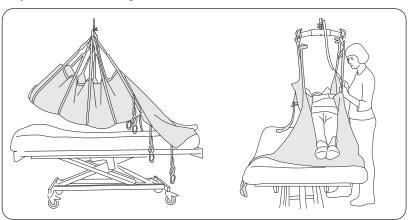
1. Connect the required number of lift straps according to earlier description above. Lift the patient free of the bed.
