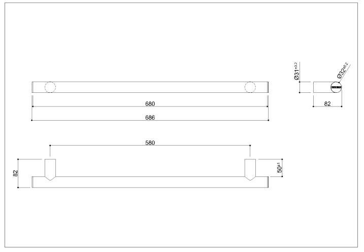
Flangeless straight safety grab rail come in a range of lengths and colours with satin finished end caps. The grab rail body is made of  $\emptyset$  32x1,5 mm stainless steel (AISI 304) tube. The internal components are made of aluminum.
