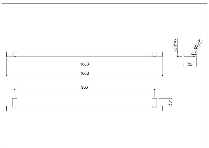
Flangeless straight safety grab rail come in a range of lengths and colours with satin finished end caps. The grab rail body is made of  $\varnothing$  32x1,5 mm stainless steel (AISI 304) tube. The internal components are made of aluminum.
