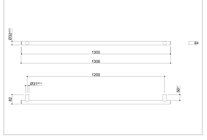
Flangeless straight safety grab rail come in a range of lengths and colours with satin finished end caps. The grab rail body is made of  $\emptyset$  32x1,5 mm stainless steel (AISI 304) tube. The internal components are made of aluminum.
