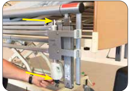
Replace the bolts and tighten one end at a time
