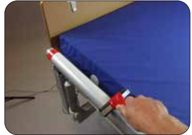
Run a hard roller over the velcro
