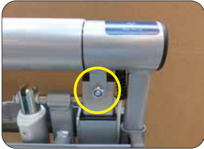
Dismount the bar from the actuator fitting
