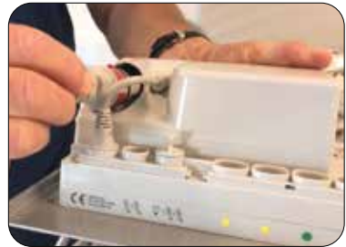
Insert the plug into the control unit
