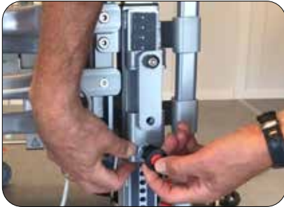
Position the bracket at the required height (can be adjusted later)
