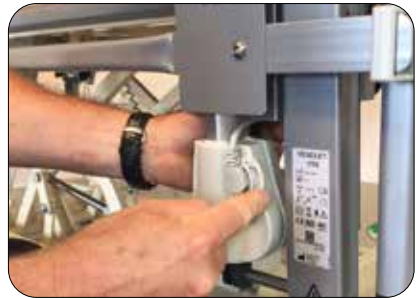
Lock the cable with the locking mechanism
