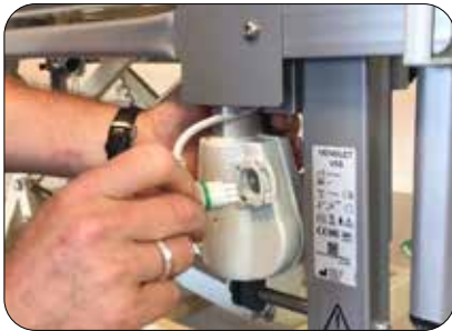
Connect the actuator cable
