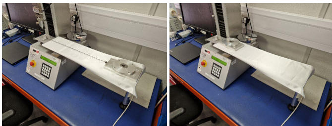
Figure 3. Tensile tester, start and end positions
