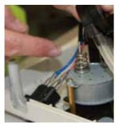
**15** Reposition the spring over the shaft, wider coils at the base (finer coils on top).
