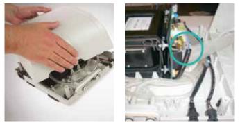
**4** Gently loosen the top and bottom housing. Once loose, hold the power socket (IEC connector) to prevent from catching while lifting the top cover and leaning it back on your work surface.
