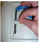
8 Insert the 'U' shaped silver bracket over the shaft, between the teeth and the plastic bracket.
