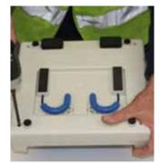
**11** Use a Phillips Head Screwdriver to replace the four screws plus washers and tighten to secure the housing together.
