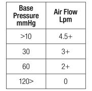
the expected pressure and air flow measurements. If air flow measurements fail to meet the specified minimum levels during any stage of the pressure test, the compressor is not operating at full capacity and needs to be replaced. Remember that a 30 minute "warm up" period is required..
