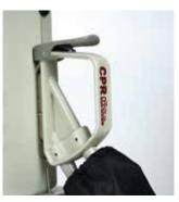
2 Check the Handle is securely attached to the Control Unit - all four connectors should be firmly inserted.
