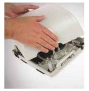
4 Gently loosen the top and bottom housing. Once loose, hold the power socket (IEC connector) to prevent from catching while lifting the top cover and leaning it back on your work surface.
