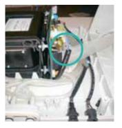
**5** Be careful not to drag the internal wires and tubing during this process. Before continuing, ensure no electrical leads are stretched and that all electrical connectors on the Printed Circuit Board (PCB) are firmly connected. You may need to prop the top housing case to prevent strain on the electrical cords.
