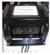
**13** Visually check that each mount is secure – gently move the compressor within the cage to ensure all mounts are connected and the compressor is correctly suspended with the metal cage.
