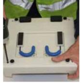
Screwdriver to replace the four screws plus washers and tighten to secure the housing together.
