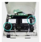
**9** Reposition the Connector Plate into the side of the control unit.
