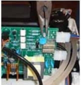
9 Using Needle Nosed Pliers, unclip the PCB from the top housing. Note the orientation of the PCB before removing it from the unit.
