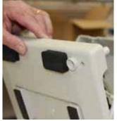
6 Lift the bottom housing up to access the base of the unit. For damaged feet, use the Needle Nose Pliers to hold the rubber base and remove from the casing.
