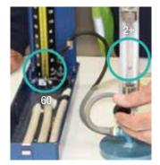
c Continue to increase back pressure resistance. Slowly close the valve on the Air Flow Meter until the Sphygmomanometer pressure reading reaches 60 mmHg. At 60 mmHg, the ball bearing inside the Air Flow Meter should drop to a minimum of 2+ litres per minute.
