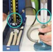
b Slowly close the valve on the Air Flow Meter to reduce airflow air and simulate 'back pressure' (i.e. to emulate the weight of a patient lying on the mattress, which forces pressure back against the flow of air from the unit). Slowly close the valve until the Sphygmomanometer pressure reading reaches 30 mmHg. At 30 mmHg, the ball bearing inside the Air Flow Meter should drop to a minimum of 3+ litres per minute.
