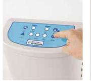
1 Switch off power supply to the Control Unit and remove the power cord from the electrical socket in the base of the unit.
