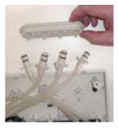
8 Unpack the replacement Connector Plate and refit all four connectors in the correct sequence, twisting clockwise to lock into place.
