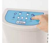
1 Switch off power supply to the Control Unit, disconnect Air Hoses and remove the power cord from the electrical socket in the base of the unit.
