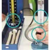
d Finish testing by fully closing the Air Flow Meter valve (maximum resistance). The ball bearing inside the Air Flow Meter should drop to 0 and the Sphygmomanometer pressure reading should rise to 120+ mmHg.
