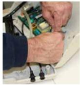
6 Trace the power lead running from underneath the synchronous motor to its connection on the circuit board. Disconnect this lead from the circuit board by carefully pulling the plastic casing (not the wiring) and gently remove the lead from under the compressor cage and leave it free.
