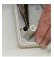
8 Once through the hole, lay the bottom housing flat and use the Needle Nose Pliers to gently pull through until the rim of the foot locks into place. Move gently from side to side while pulling, rather than applying direct upward force, to avoid snapping the nose of the replacement foot.
