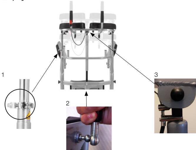
Ensure that the arm supports are raised to the maximum height, that the gas spring is fully extended and that the locking clamps (1) are locked before removing the gas spring.
