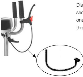
Disconnect the cable set by first loosen the adjustment screw on the cable and secondly unhook the cable from the bracket. Attach the new cable set to the old one, while still mounted in the frame, and change the old cable by pulling the cable through the frame. Ensure correct mounting and adjustment by function control.
