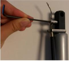
Use an Allen key to release the adjustment cable from the gas spring release head.
