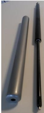
The gas spring release head is removed and the gas spring can then be removed from the gas spring tube and replaced.
