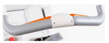
The perceptive and ergonomic handle is equipped with load cells that intercepts your every move. By gently pushing it, EvaDrive moves forward. By pulling it lightly, EvaDrive reverses.
